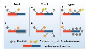
Scheme 1 Models of multicomponent electrocatalysts.
