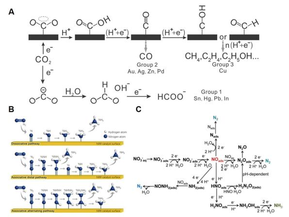
Fig. 2 (A) The possible pathways of multi-step activation and transformation of CO2 to various value-added products. Reprinted with permission from ref. 15. Copyright 2016, John Wiley & Sons, Inc.; Proposed roadmap of multi-step electroreduction of (B)  $N_2$  and (C)  $NO_3^-$  towards  $NH_3$ synthesis. Reprinted with permission from ref. 22 and 23. Copyright 2019, Elsevier and Copyright 2021, the Royal Society of Chemistry.
