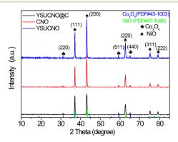
Fig. 1 XRD patterns of the YSUCNO, YSUCNO@C, and CNO microspheres.
