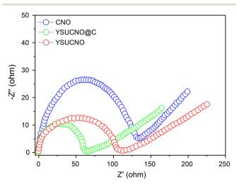
Fig. 5 Impedance patterns of the YSUCNO, YSUCNO@C, and CNO microspheres.
