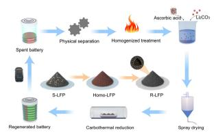
Fig. 1 Schematic illustration of the regeneration process of spent LFP.
