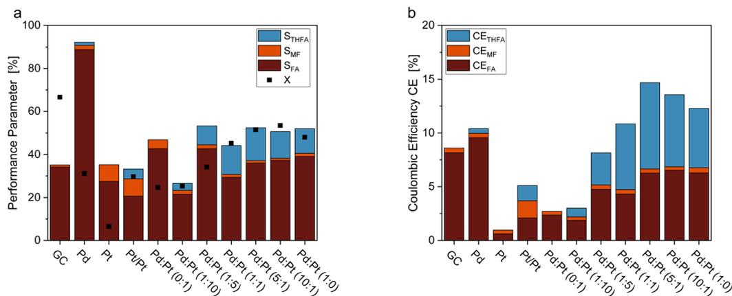
**Fig. 3** Comparison of different working electrodes for their reaction performance indicators (a) X and S, (b) CEs), including metal sheet electrodes (Pd, Pt), platinumized platinum sheet (Pt/Pt), and Glassy Carbon (GC) electrodes coated with catalytic inks containing varying Pd : Pt ratios. With 0.05 M FF solution in 0.5 M H<sub>2</sub>SO<sub>4</sub> electrolyte with 15% acetonitrile under galvanostatic conditions with –300 mA, and 6 FEq transferred electrons.
