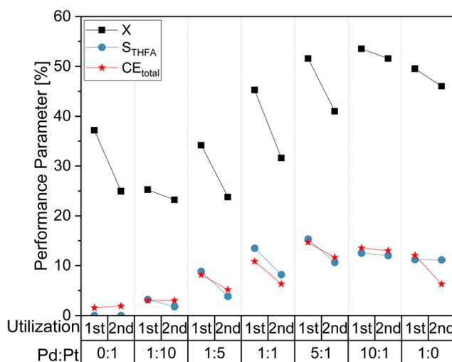
Fig. 4 Comparison of selected reaction performance parameters for the first and second utilization of different electrode material compositions. With 0.05 M FF solution in 0.5 M  $\text{H}_2\text{SO}_4$  electrolyte with 15% acetonitrile under galvanostatic conditions with  $-300$  mA and 6 FEq transferred electrons.
