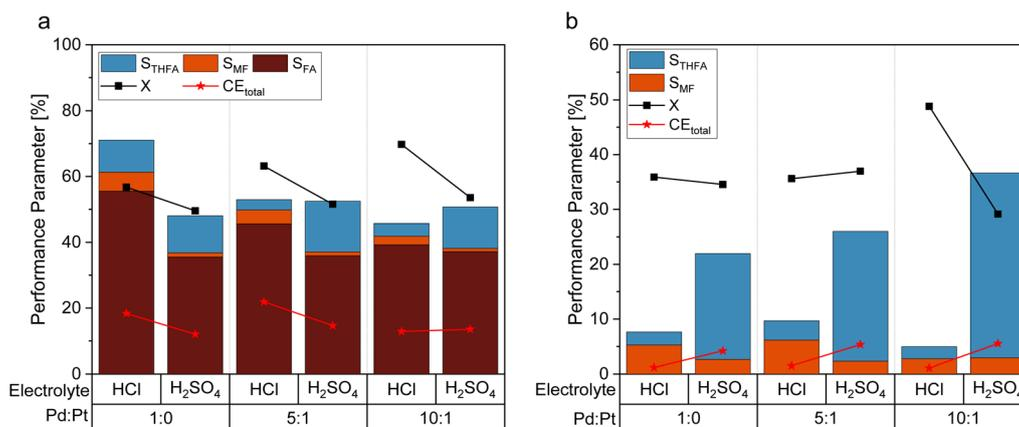
Fig. 5 Comparison of selected reaction performance parameters for the utilization of 0.5 M HCl solution and 0.5 M  $\text{H}_2\text{SO}_4$  solution with 15% acetonitrile for the utilization of (a) furfural and (b) furfuryl alcohol as starting material with 0.05 M FF solution under galvanostatic conditions with  $-300$  mA and 6 FEq transferred electrons.
