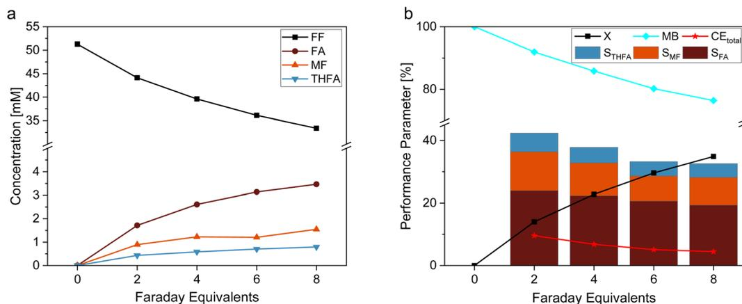
**Fig. 2** (a) Concentration profile and (b) reaction performance parameters of the hydrogenation reaction of FF on platinumized platinum (Pt/Pt) electrodes under variation of the total amount of transferred charge with 0.05 M FF solution in 0.5 M H<sub>2</sub>SO<sub>4</sub> electrolyte with 15% acetonitrile under galvanostatic conditions with –300 mA.
