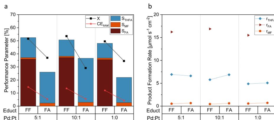
**Fig. 6** Comparison of FF and FA as starting material with selected Pd:Pt on GC electrodes. (a) Reaction performance parameters and (b) product formation rates. With 0.05 M FF respectively FA solution in 0.5 M H<sub>2</sub>SO<sub>4</sub> electrolyte with 15% acetonitrile under galvanostatic conditions with –300 mA and 6 FEq transferred electrons.
