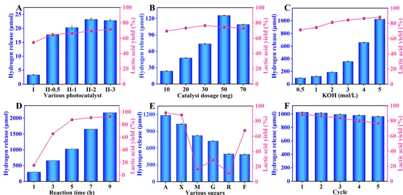
Fig. 4 The effects of various conditions on co-production of hydrogen and lactic acid, (A) different photocatalysts (I: CN, II: RuS<sub>2</sub>@CN), (B) catalyst dosages (5.0 h, 30 °C), (C) KOH concentrations (10.0 mg RuS<sub>2</sub>@CN-2, 5.0 h), (D) irradiation time (10 mg RuS<sub>2</sub>@CN-2, 5.0 M KOH). (E) The selective oxidation of different biomass-derived sugars to hydrogen and lactic acid photocatalyzed by RuS<sub>2</sub>@CN-2. (F) Recycling test of RuS<sub>2</sub>@CN-2.
