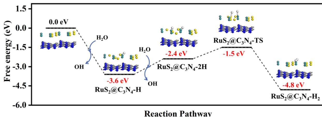
Fig. 7 The hydrogen generation pathway calculated by DFT.
