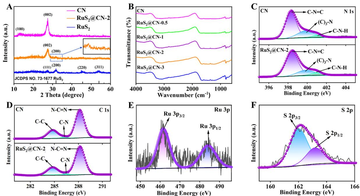
Fig. 2 XRD patterns of CN,  $\text{RuS}_2\text{@CN-}2$ , and  $\text{RuS}_2$  (A). FT-IR spectra of as-prepared samples (B). XPS high-resolution spectra of CN and  $\text{RuS}_2\text{@CN-}2$ : N 1s (C), C 1s (D), Ru 3p (E) and S 2p (F).
