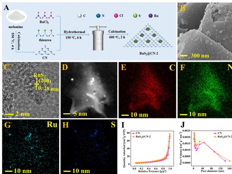
Fig. 1 Preparation scheme of  $\text{RuS}_2\text{@CN-}x$  (A). SEM image (B) and TEM images (C and D) of  $\text{RuS}_2\text{@CN-}2$ . Elemental mapping images of  $\text{RuS}_2\text{@CN-}2$ : C (E), N (F), Ru (G), S (H).  $\text{N}_2$  adsorption–desorption isotherms of CN and  $\text{RuS}_2\text{@CN-}2$  (I). Pore width distribution of CN and  $\text{RuS}_2\text{@CN-}2$  (J).
