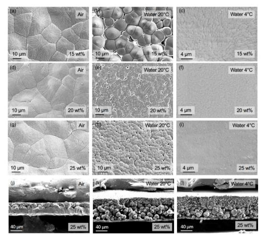
Fig. 4 Surface morphology of pure PP membranes prepared with 15 wt% (a–c), 20 wt% (d–f), and 25 wt% (g–i) PP solutions in  $\alpha$ -pinene and quenched in air at room temperature (a, d and g), water at 20 °C (b, e and h), and water at 4 °C (c, f and i); cross-section images of membranes prepared from 25 wt% PP solutions in  $\alpha$ -pinene quenched under different conditions (j–l).
