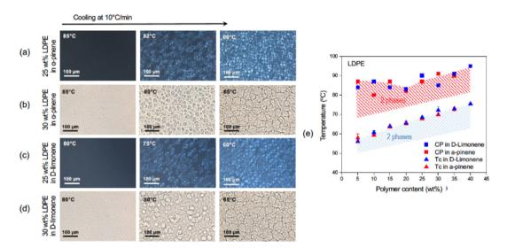
Fig. 3 (a and c) Polarized and (b, d) non-polarized optical microscopy cloud point (CP) measurements; (e) corresponding phase diagram obtained by cloud point and DSC crystallization ( $T_c$ ) measurements for LDPE in α-pinene and p-limonene.
