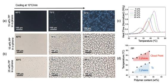
Fig. 2 (a) Polarized and (b) non-polarized optical microscopy cloud point (CP) measurements; (c) crystallization ( $T_c$ ) measurement by DSC temperatures for PP in α-pinene; and (d) corresponding phase diagram.
