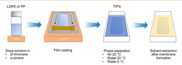
Fig. 1 Schematic of polymeric membrane preparation via TIPS: preparation of the dope solution containing the polymer and the solvent, casting of the solution on a stainless steel plate, phase separation of the membrane by quenching media at a temperature below the crystallization temperature, and solvent extraction in ethanol.
