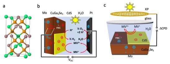
Fig. 1 (a) Crystal structure of  $CuGaSe_2$ , the parent phase of  $CuGa_3Se_5$ , (b) PEC cell, (c) liquid SPV configuration. MV = methylviologen.
