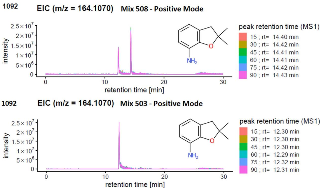
Fig. 4 Extracted Ion Chromatogram (EIC) of  $m/z$  161.1070 in (top) mix 508 and (bottom) mix 503. In mix 503 only one compound with this mass is present (level 1), but another isobaric compound is present in mix 508.
