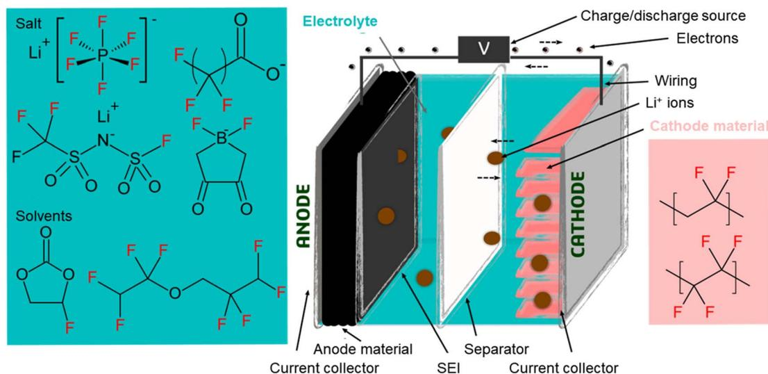
**Fig. 1** Simplified schematic of a lithium-ion battery, adapted from Bresser *et al.* (2015),<sup>38</sup> including examples of fluorinated species included in many batteries, some of which are classified as PFAS under the OECD definition.
