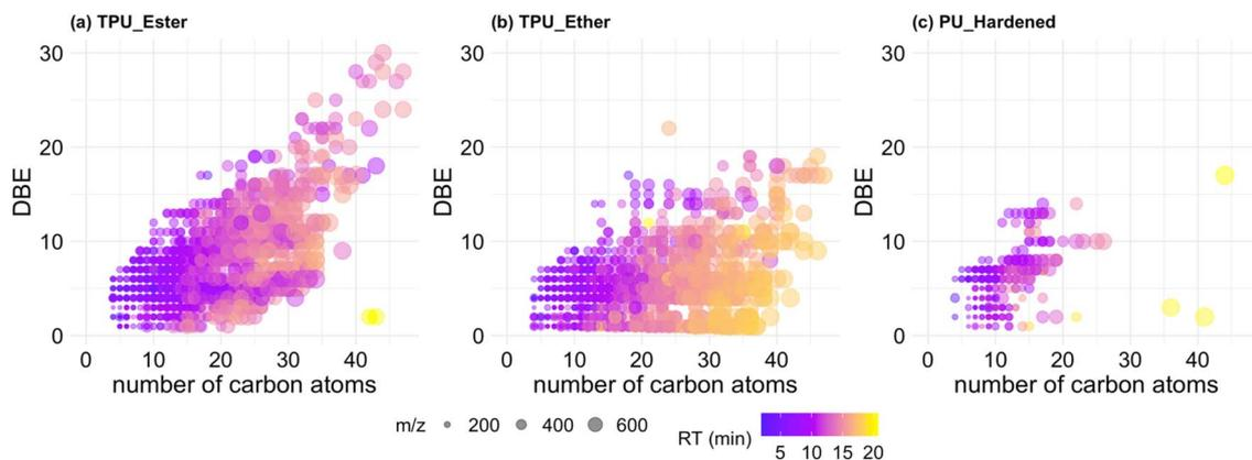
Fig. 5 Double-bond-equivalence (DBE) versus number of carbon atoms of all formula-annotated features detected in TPU\_Ester (a), TPU\_Ether (b), and PU\_Hardened (c). Each data point represents an annotated formula. Data point marker size represents feature size expressed as mass-to-charge ( $m/z$ ) value. The color scale represents feature retention time (RT) in minutes.
