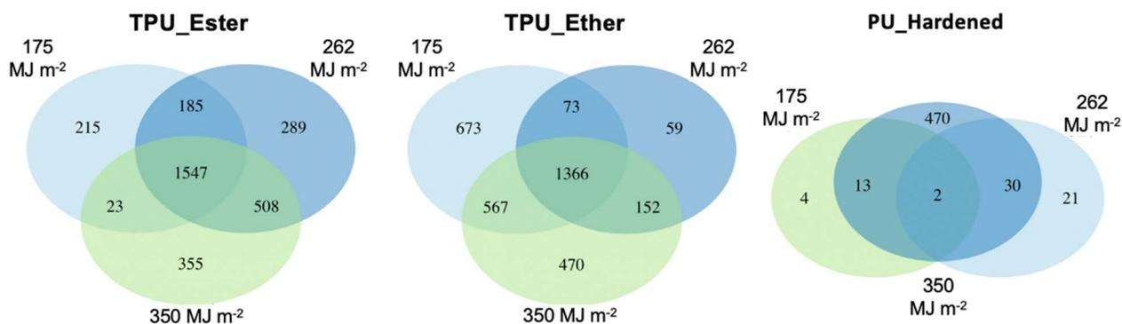
Fig. 3 Venn diagrams of feature distribution in TPU\_Ester (left), TPU\_Ether (center), and PU\_Hardened (right) irradiated with a UV dose of 175, 262 and 350 megajoule per square meter ( $\text{MJ m}^{-2}$ ).
