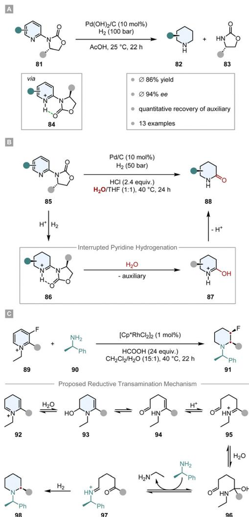
**Scheme 14** Chiral auxiliary assisted asymmetric hydrogenations of pyridines and pyridinium salts.<sup>108,110,112</sup>
