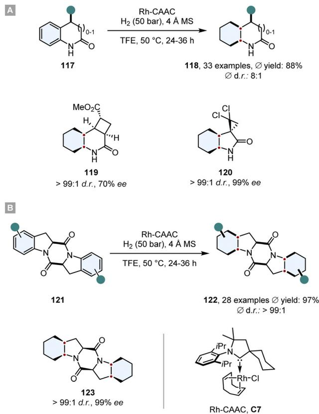
**Scheme 17** Asymmetric diastereoselective hydrogenations of (A) 2-oxindoles, 3,4-dihydroquinolones and (B) aromatic 2,5-diketopiperazines with a highly selective Rh-CAAC catalyst.<sup>124,125</sup>
