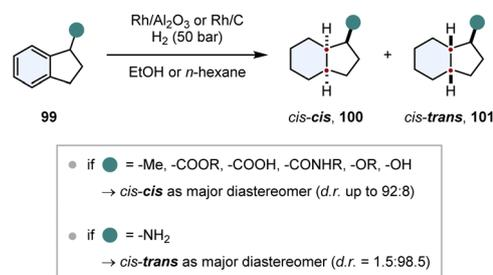
**Scheme 15** Investigation of substituent effects on the diastereoselective hydrogenation of 1-substituted indanes.<sup>117,118</sup>
