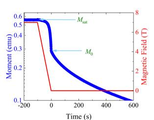
Fig. 3 Example DC decay measurement. Samples are saturated at high magnetic field before the field is swept to the target field. In a Quantum Design MPMS3 the fastest field sweep rate is 700 Oe s<sup>-1</sup>, such that it takes  $\approx 100$  s to go from 7 T to 0 T. The *x*-axis is set to t = 0 s at  $M_0$ , and  $M_{eq}$  is not shown on this scale.
