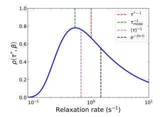
Fig. 2 Distribution of the stretched exponential function with  $\tau^* = 1$  s and  $\beta$  = 0.6 showing the four measures of the rate:  $\tau^{\star -1}$ ,  $\tau_{\text{mode}}^{-1}$  (eqn (7)),  $\langle \tau \rangle^{-1}$ (eqn (8)<sup>15</sup>),  $e^{-\langle ln[\tau] \rangle}$  (eqn (9)<sup>26</sup>).
