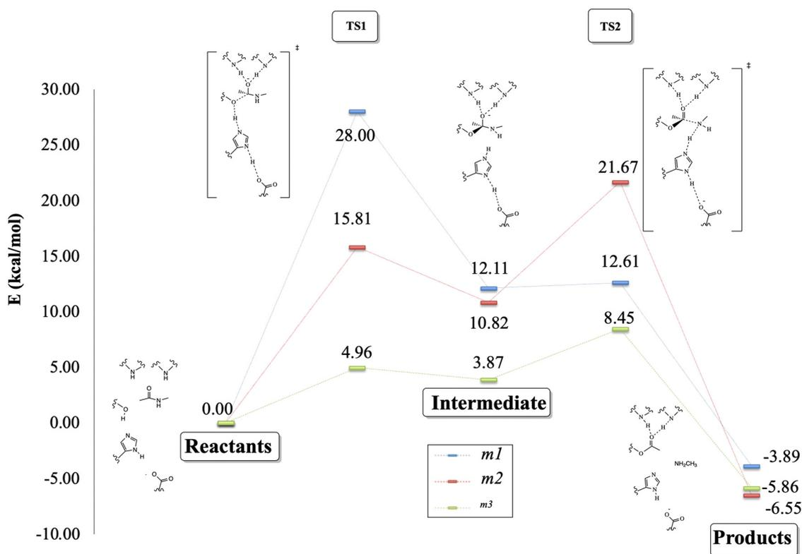
Fig. 7 Proposed reaction mechanism ( $\text{kcal mol}^{-1}$ ) for the peptide bond rupture. In blue is shown the reaction path for the **m1** model, in red are shown the results for **m2** and in green are shown the results obtained for **m3**.
