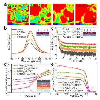
**Fig. 2** (a) Confocal PL mapping images, (b) PL spectra, and (c) TRPL spectra of the control and 7-Al derivative modified perovskite films directly deposited on the glass substrate. (d) SCLC curves of the electron-only device with a structure of  $FTO/SnO_2-TiO_xCl_{4-2x}/perovskite/PCBM/carbon without and with 7-Al derivative treatment. (e) Mott–Schottky (M–S) of various devices with a structure of <math>FTO/SnO_2-TiO_xCl_{4-2x}/perovskite/carbon$ .
