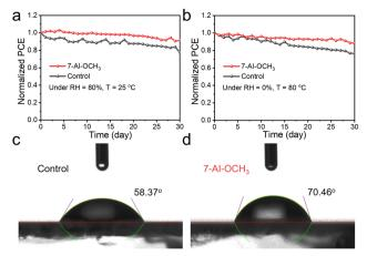
Fig. 4 Long-term stability of the inorganic CsPbBr<sub>3</sub> PSCs at (a) RH = 80%T = 25 °C and (b) RH = 0%, T = 80 °C. The water contact angle of (c) control and (d) 7-AI-OCH<sub>3</sub>-based perovskite films.
