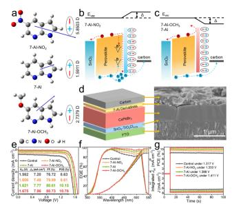
Fig. 3 (a) Calculated dipole moment images of the three molecules. Schematic illustration of charge carrier collection and recombination in (b) 7-AI-NO $_2$ -based PSCs and (c) (AI or AI-OCH $_3$ )-based PSCs. (d) The architecture and cross-sectional SEM image of all-inorganic CsPbBr $_3$  PSCs. (e) The J-V curves, (f) IPCE spectra, and (g) steady power output curves of various CsPbBr $_3$  PSCs.
