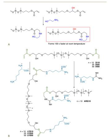
(A) Acceleration of the aza-Michael reaction with proximal OH groups that, <sup>66</sup> (B) allow the synthesis of amino acid-modified silicones. <sup>43</sup>
