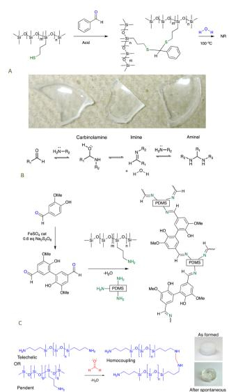
(A) Crosslinking thiopropylsilicones with aldehydes.<sup>67</sup> Photo from ref. 67 reproduced with permission from the Royal Society of Chemistry. (B) Reactions between aldehydes and amines. (C) Schiff base crosslinks, 69 and (D) aminal-based crosslinks from aminosilicones.71
