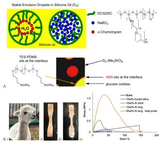
Fig. 14 (A) Enzyme-containing water-in-silicone oil emulsions. 97,108 Scheme and photo from ref. 97 and 108 reproduced with permission from the American Chemical Society. (B) (i) Alpaca, silicone elastomer containing (ii) 10 wt% short and (iii) 10 wt% long alpaca fibers, (iv) enormous difference in materials properties based on fiber length at the same mass loading. 100 Photographs from ref. 100 reproduced with permission from the Royal Society of Chemistry.
