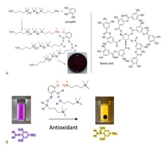
(A) Formation of elastomers simply by mixing aminosilicones with phenols. (B) Antioxidant activity of the elastomer formed. 70 Photographs from ref. 70 reproduced with permission from the American Chemical Society.
