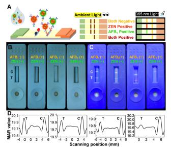
Fig. 2 (A) A diagram illustrating the production process of multiplexed ICTS for co-detection of ZEN and AFB<sub>1</sub>. (B) Photographs of test strips after interacting with sample solutions containing varying concentrations of AFB<sub>1</sub> and ZEN. Their corresponding (C) fluorescence images under UV light and (D) magnetic signals. The AFB<sub>1</sub>/ZEN concentrations in (B-D) are as follows (from left to right): 0/0, 150/0, 0/150, 150/150 ng mL<sup>-1</sup>.
