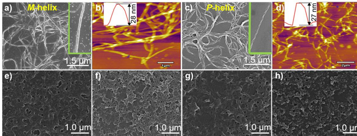
Fig. 2 SEM and AFM images of supramolecular structures of (a and b)  $\text{Ag}^+-\text{L}-1$  formed in THF, and (c–h)  $\text{Ag}^+-\text{D}-1$  in (c and d) THF, (e) EtOH, (f) MeOH, (g)  $\text{CH}_3\text{CN}$  and (h)  $\text{H}_2\text{O}$ . The insets in (a) and (c) show, respectively, two types of polymeric structures, namely the *M*-helix of  $\text{Ag}^+-\text{L}-1$  and *P*-helix of  $\text{Ag}^+-\text{D}-1$ .  $[\text{Ag}^+-\text{L}-1] = [\text{Ag}^+-\text{D}-1] = 25 \mu\text{M}$ .
