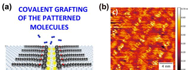
**Fig. 12** (a) Scheme of the covalent grafting of patterned molecules on the surface of graphene. (b) STM height image of molecules self-assembled on graphene. Reproduced with permission.<sup>46</sup> Copyright 2016, American Chemical Society.
