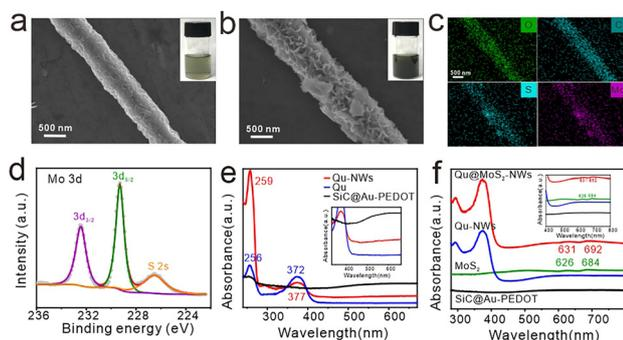
**Fig. 1** (a) SEM image of a Qu-NW (inset: the digital image of the Qu-NW dispersion). (b) SEM image of a Qu@MoS<sub>2</sub>-NW (inset: the digital image of the Qu@MoS<sub>2</sub>-NW dispersion) and (c) corresponding SEM-EDX elemental mapping images. (d) XPS data of Mo 3d states from Qu@MoS<sub>2</sub>-NWs. (e and f) UV/Vis absorption of Qu-NWs, Qu, SiC@Au-PEDOT NWs, Qu@MoS<sub>2</sub>-NWs and MoS<sub>2</sub>.
