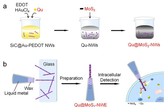
**Scheme 1** Illustration of (a) the large-scale synthesis of Qu and MoS<sub>2</sub> co-functionalized nanowires and (b) the preparation of nanosensors for the electrochemical detection of intracellular hydrogen sulfide.
