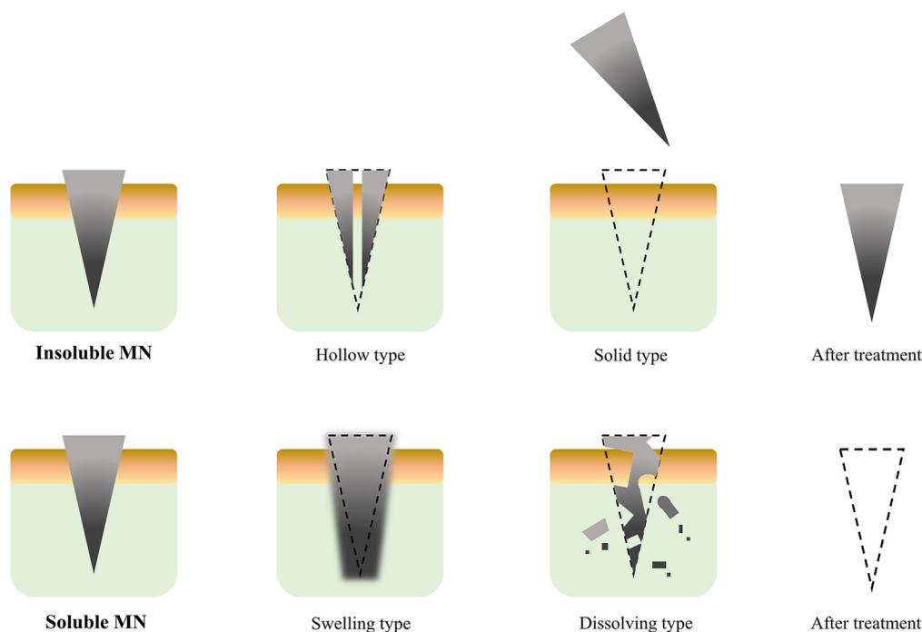
Fig. 8 Classification of microneedle system: insoluble type and soluble type.
