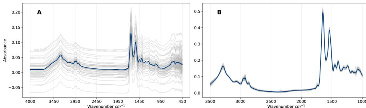
**Fig. 1** (A) 50 randomly selected raw spectra from dataset A in the frequency domain (representation  $F_R$ ) (grey) and the corresponding mean spectrum (blue). (B) Same subset of EMSC pre-processed spectra (representation  $F$ ) (grey) and corresponding mean spectrum (blue).
