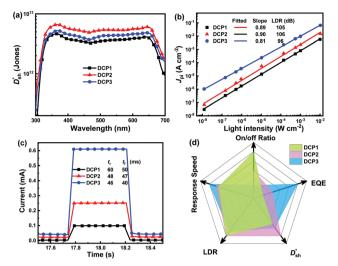
Fig. 4 Single-polymer DCP1-, DCP2-, and DCP3-based PM-OPDs: (a)  $D_{\mathrm{sh}}^{*}$  spectra, (b) LDR analysis, (c) transient photocurrents of PM-OPDs under a bias of 10 V, and (d) radar map analysis of the key parameters.
