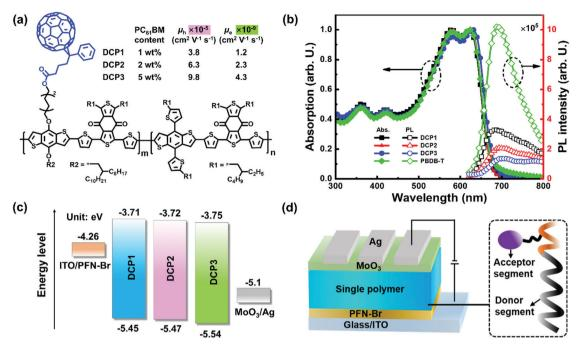
Fig. 1 (a) The chemical structures of the polymers. (b) Absorption and PL spectra of PBDB-T and polymer films. (c) Energy levels of the polymers, ITO/ PFN-Br, <sup>23</sup> and the  $MoO_3/Ag$  electrode. (d) The device architecture of a PM-OPD with a single polymer as the active layer.
