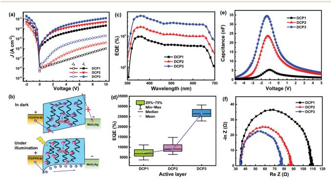
Fig. 2 (a) J-V curves of all PM-OPDs under dark and light-illumination conditions. (b) Schematic diagrams of the working mechanism of the PM-OPD. (c) The EQE spectra of all PM-OPDs under a bias of 10 V. (d) EQE box plots of all PM-OPDs; Max: maximum, Min: minimum. (e) C-V curves and (f) Nyquist plots of all PM-OPDs.
