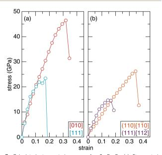
Fig. 7 Calculated stress–strain curves for  $Sc_2Ru_5B_4$  (a) Stress–strain curves for various crystallographic directions under applied tension. (b) Stress–strain curves for the hardest and softest shear systems.
