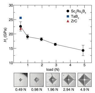
Fig. 2 Vickers microindentation (H<sub>V</sub>) measurements of Sc<sub>2</sub>Ru<sub>5</sub>B<sub>4</sub> from low (0.49 N) to high (4.9 N) load and  $TaB_2$  and ZrC at low (0.49 N) load. Error bars correspond to the average error of multiple independent measurements. Representative indentations from each applied load are shown below the plot.
