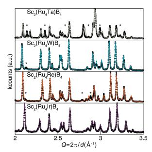
Fig. 5 Powder X-ray diffractograms of the solid solution Sc<sub>2</sub>(Ru<sub>4</sub>TM)B<sub>4</sub> (TM = Ta, W, Re, and Ir) and the associated Le Bail refinements.
