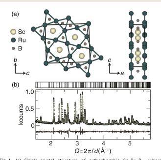
Fig. 1 (a) Single-crystal structure of orthorhombic  $Sc_2Ru_5B_4$ , where scandium is cream, ruthenium is teal, and boron is dark gray shown along the a-direction (left) and along the b-direction (right). (b) Le Bail refinement of  $Sc_2Ru_5B_4$ . Black circles represent the measured data, the refinement fit is in cream and the black line represents the difference.
