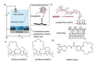
**Fig. 6** (a) Schematic of the OECT device, employing the poly(EDOTOA-co-EDOT)/PEDOT:PSS composite as the active channel material. (b) Chemical structure of the 2,6-sialyllactose functionalized EDOT derivative. Reproduced from ref. 72 with permission from Elsevier. (c) Chemical structures of crown ether functionalized **PEDOT** copolymer. <sup>73</sup> (d) Chemical structure of **PEDOT-Crown.** <sup>74</sup>
