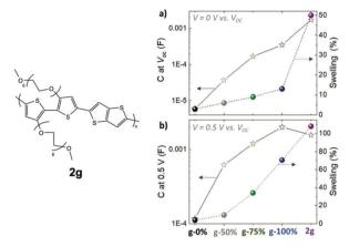
Fig. 11 The swelling behaviour and volumetric capacitance with respect to different glycol fractions in p(g2T-TT) and 2g based polymers at (a) V =0 V and (b) V = 0.5 V versus  $V_{OC}$ . Reproduced from ref. 79 with permission from Wiley-VCH.
