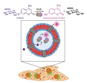
Fig. 1 Schematic representation of the catalytic nanocompartment containing GUS and its enzymatic activity. Melittin pores in the PDMS<sub>25</sub>b-PMOXA<sub>10</sub> membrane provide a pathway to from the compartment interior where β-glucuronidase (GUS) catalyses the production of hymecromone (4-MU) from its glucuronide conjugate (4-MUG) within cells that have taken up CNCs.
