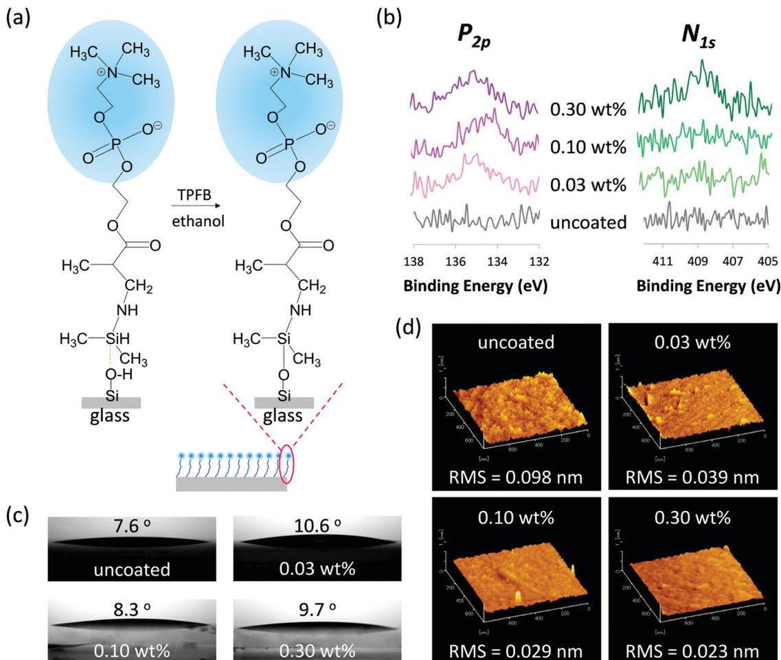
**Fig. 3** Formation and characterization of MPC-Si coatings on glass substrates. (a) Schematic drawing of self-assembly of MPC-Si molecules on the glass substrates via the silanization reaction to form MPC-Si coatings. (b) XPS spectra of phosphorus ( $P_{2p}$ ) and nitrogen ( $N_{1s}$ ), (c) water contact angle images, and (d) AFM images of the glass substrates coated with the 0.03 wt%, 0.10 wt%, and 0.30 wt% MPC-Si in comparison with those of uncoated glass substrates.
