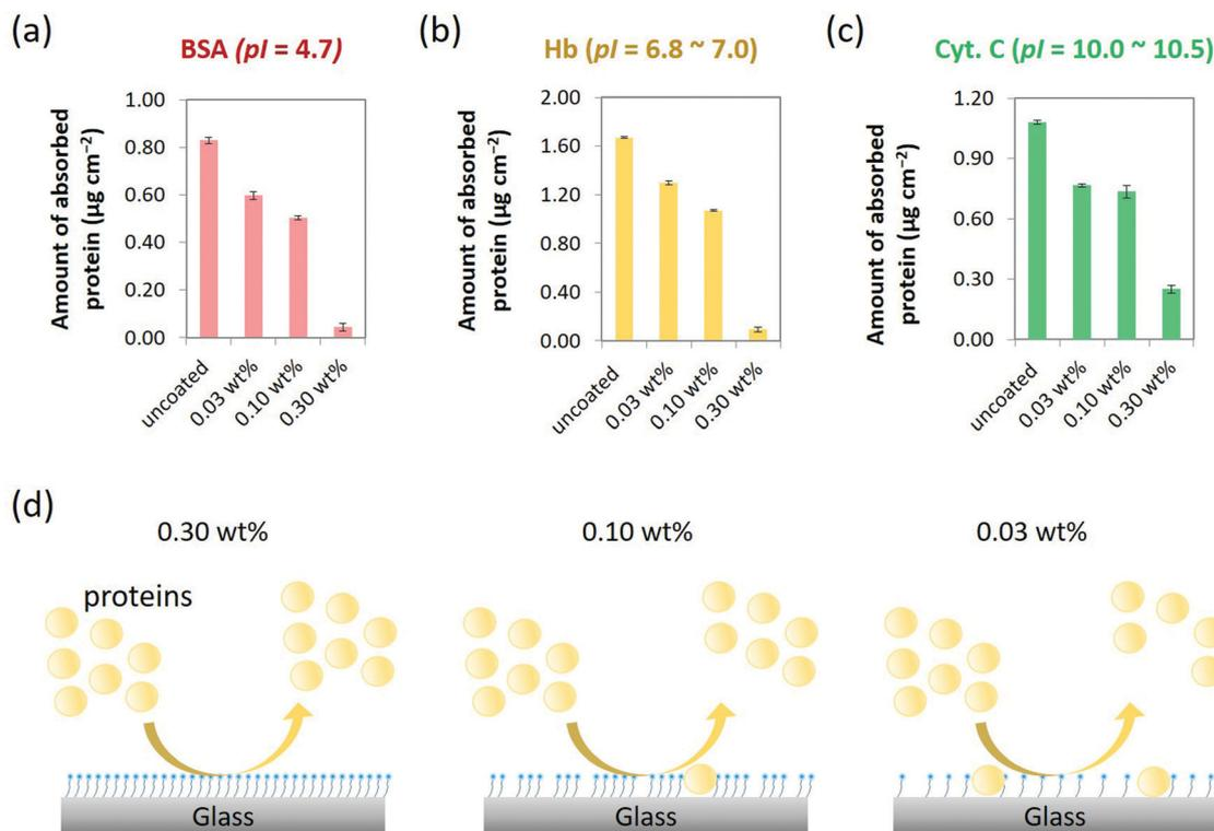
Fig. 4 Amounts of typical (a) anionic (BSA), (b) neutral (Hb), and (c) cationic (Cyt. *c*) proteins adsorbed on the glass substrates coated with the 0.03 wt%, 0.10 wt%, and 0.30 wt% MPC-Si in comparison with those of uncoated glass substrates. (d) Different NPA suppressing capabilities exhibited by MPC-Si coatings of different concentrations, which may be ascribed to the difference in the density of the MPC-Si molecules on the surface.
