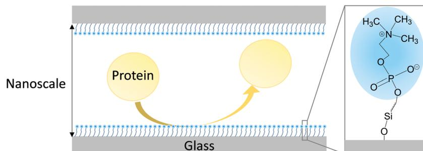
Fig. 1 Conceptual drawing of the MPC-Si coating enabling suppression of non-specific protein adsorption in a nanofluidic channel.
