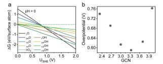
Fig. 5 DFT calculations on  $IrO_2(110)$ . (a) Surface phase diagram of  $IrO_2$  at pH=0. (b) Theoretical overpotential of the defective  $IrO_2$  surface with different GCNs.
