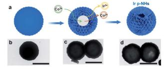
Fig. 1 (a) Schematic illustration of the structural evolution of Ir p-NHs, with corresponding TEM images of products collected at a reaction time of (b) 1 h, (c) 3 h and (d) 5 h. Scale bar, 1  $\mu$ m.
