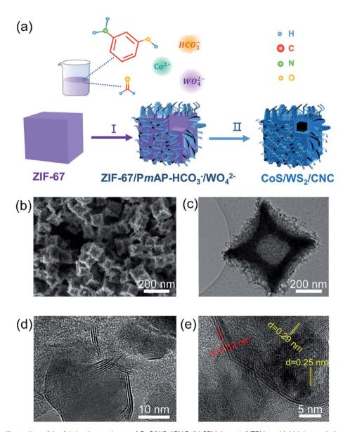
Fig. 1 (a) Schematic illustration of the fabrication pathway of CoS/WS<sub>2</sub>/CNC. (b) SEM, (c and d) TEM, and (e) high-resolution TEM images of CoS/ WS<sub>2</sub>/CNC-1.
