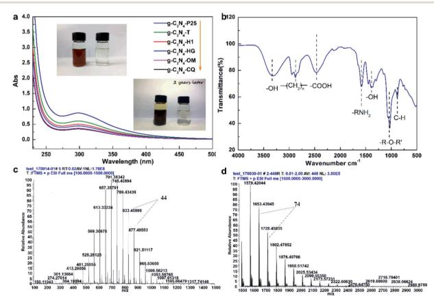
Fig. 4 Aqueous triethanolamine (TEOA) polymerization by STAP. (a) UV-Vis absorption spectrum. Inset: the photograph of colorless TEOA (left) and brown polymeric products in water (right). (b) FTIR spectrum. (c) Typical mass spectrum for small molecular weight. (d) Typical mass spectrum for large molecular weight.
