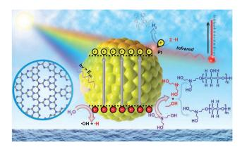
Scheme 1 Schematic illustration of heterogeneous solar thermalactivated photocatalysis (STAP) for hydrogen (H2) production and agueous triethanolamine (TEOA) polymerization.
