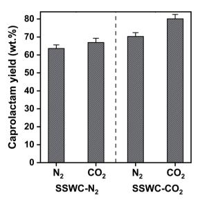
Fig. 8 Caprolactam yield from the thermocatalytic conversion of FNW at  $500\,^{\circ}$ C under  $N_2$  and  $CO_2$  environments using SSWC- $N_2$  and SSWC- $CO_2$  in an *in situ* catalyst configuration.
