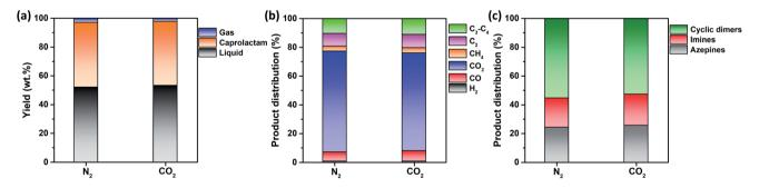
Fig. 3 (a) Yields of gaseous and liquid products, and caprolactam produced from the non-catalytic thermal conversion of FNW at 500  $^{\circ}$ C under N<sub>2</sub> and CO<sub>2</sub> environments; (b) distribution of gaseous products; (c) distribution of liquid products.
