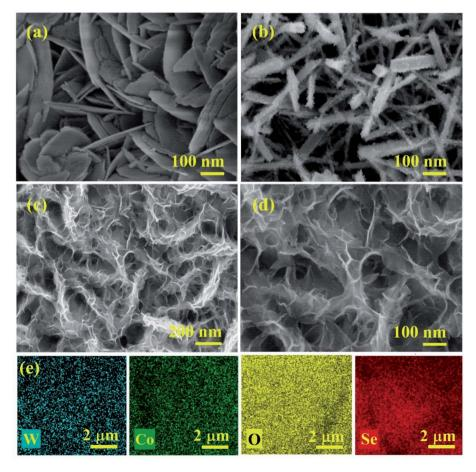
Fig. 1 FE-SEM images of (a) WSe<sub>2</sub>/WO<sub>2</sub> and (b) CoSe/Co<sub>3</sub>O<sub>4</sub>, (c) low and (d) high magnification images of the WCoSe/WCo<sub>3</sub>O<sub>4</sub> heterostructure, and (e) EDS color mapping with the corresponding elements of W, Co, O, and Se of the WCoSe/WCo<sub>3</sub>O<sub>4</sub> heterostructure.
