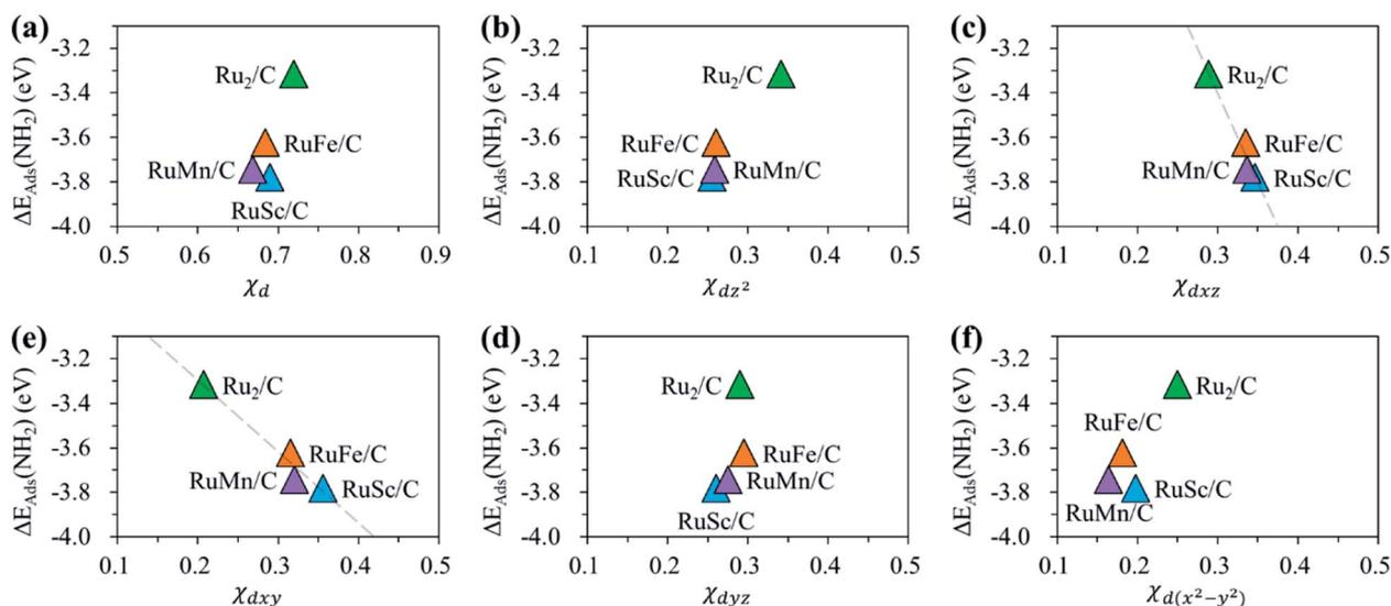
Fig. 11 Relationship between  $\text{NH}_2$  adsorption energy [ $\Delta E_{\text{ads}}(\text{NH}_2)$ ] and orbital overlap [ $\chi_d$ ] for the RuM (M = Sc, Mn, Fe) DACs (a)  $\chi_d$ , (b)  $\chi_{d_{z^2}}$ , (c)  $\chi_{d_{xz}}$ , (d)  $\chi_{d_{xy}}$ , (e)  $\chi_{d_{xy}}$  and (f)  $\chi_{d_{x^2-y^2}}$ .
