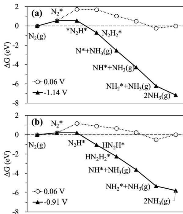
Fig. 3 Calculated free energy profiles at equilibrium (○) and limiting (▲) potentials for the  $\text{N}_2\text{RR}$  on (a) the Ru SAC and (b) the homo- $\text{Ru}_2$  DAC via the most favourable pathway.
