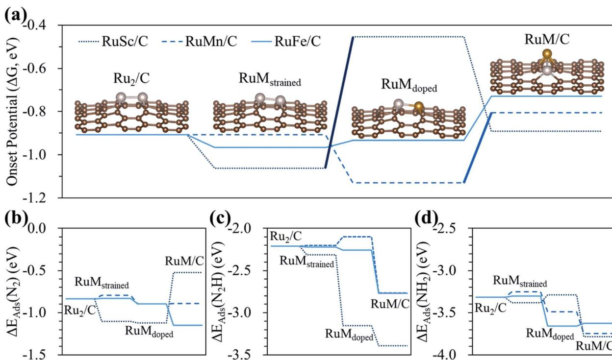
Fig. 8 Contribution of strain, dopant and configurational effects to the (a) onset potential, and adsorption energy of (b)  $N_2$ , (c)  $N_2H$ , and (d)  $NH_2$  of the  $N_2$ RR on the hetero- $RuM$  DACs. In (a), the bold solid lines indicate the change in the limiting step from  $[N_2^* + (H^+ + e^-) \rightarrow N_2H^*]$  to  $[NH_2^* + (H^+ + e^-) \rightarrow NH_3(g)]$ .
