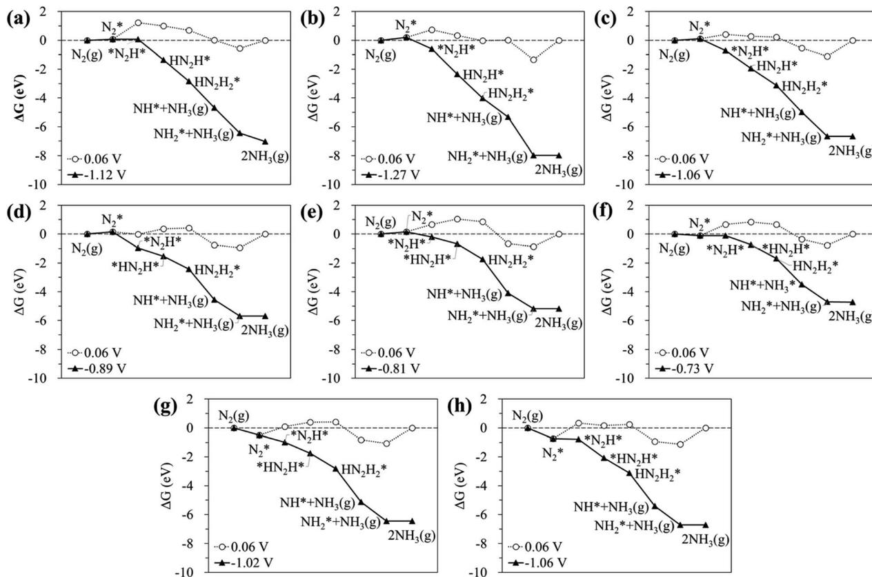
Fig. 6 Calculated Gibbs free energy profiles at equilibrium (O) and limiting ( $\blacktriangle$ ) potentials for the  $N_2$ RR on hetero-RuM DACs of group I [(a) RuTi/C, (b) RuV/C, and (c) RuCr/V], group II [(d) RuSc/C, (e) RuMn/C, and (f) RuFe/C], and group III [(g) RuCo/C and (h) RuNi/C] via the most favourable pathway.
