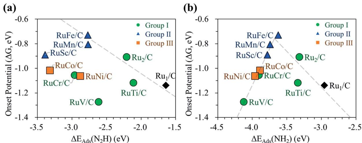
Fig. 7 Relationship between the onset potential of the  $N_2$ RR and the adsorption energies of (a)  $N_2H$  and (b)  $NH_2$ . In (b), the PLS of the catalysts located on the left side of the peak position is (5)  $NH_2^* + (H^+ + e^-) \rightarrow NH_3(g)$ , while for the right-side case, the PLS is (6)  $N_2^* + (H^+ + e^-) \rightarrow N_2H^*$ .
