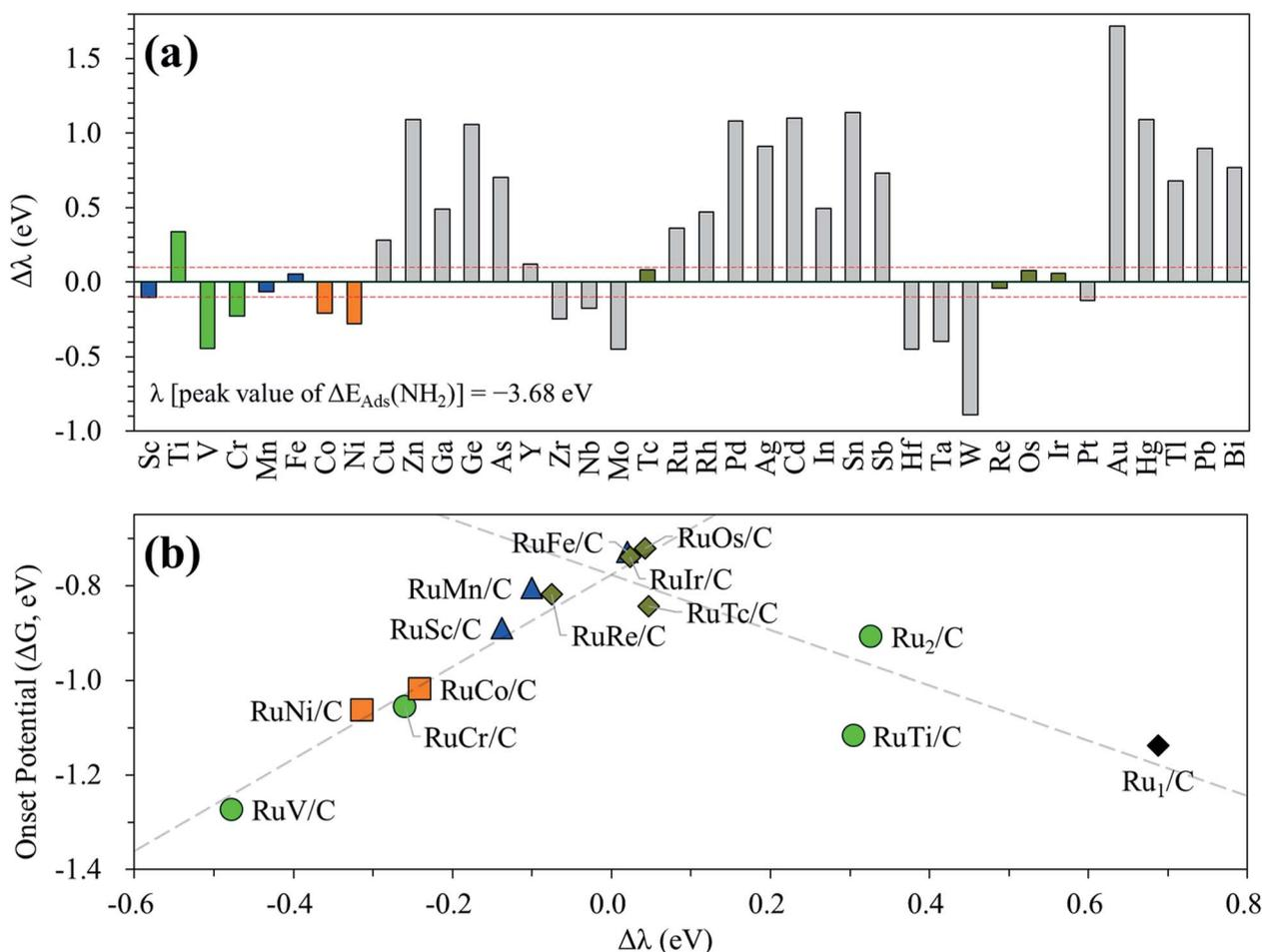
Fig. 12 (a) Screening results using NH<sub>2</sub> adsorption energy as a descriptor in RuM/C, in which M is extended to 4d, 5d, 5p, and 6p elements, and (b) revised volcano plot by adding four more candidates. In (b), the PLS of the catalysts located on the left leg of the peak position is [(5) NH<sub>2</sub>\* + (H<sup>+</sup> + e<sup>-</sup>) → NH<sub>3</sub>(g)], while for the right leg case, the PLS is [(6) N<sub>2</sub>\* + (H<sup>+</sup> + e<sup>-</sup>) → N<sub>2</sub>H\*].
