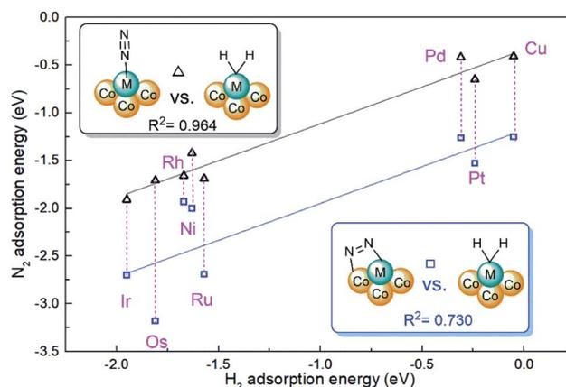
Fig. 4 Relationship between  $N_2$  adsorption and  $H_2$  adsorption on  $M_1Co_n/CoO_x$  SCCs.
