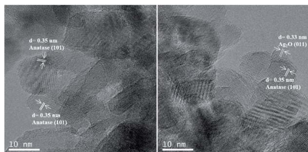
Fig. 2 TEM images of In-TiO<sub>2</sub>-1 (left) and Ag/In-TiO<sub>2</sub>-1 (right).
