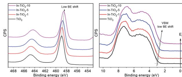
Fig. 5 XPS of In-doped  $TiO_2$  samples in the Ti 2p<sub>3/2</sub> (left) and VB (right) regions.
