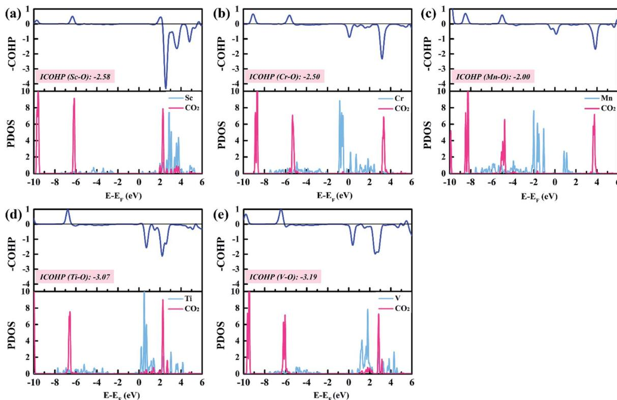
Fig. 8 The PDOSs and COHPs of CO<sub>2</sub> on TM@Na<sub>4</sub>SiMo<sub>12</sub> (TM = Sc, Cr, Mn, Ti and V).
