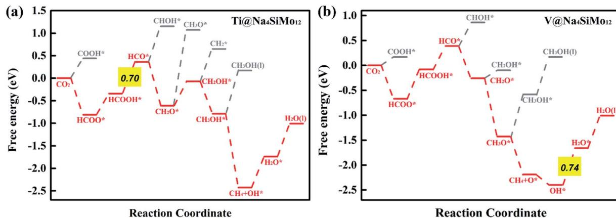
Fig. 7 Calculated free energy diagrams for the electrochemical CO<sub>2</sub>RR on (a) Ti and (b) V@Na<sub>4</sub>SiMo<sub>12</sub>.
