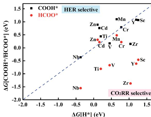
Fig. 4 Free energy change ( $\Delta G$ ) of the first protonation step in the CO<sub>2</sub>RR and HER on TM@Na<sub>4</sub>SiMo<sub>12</sub>.
