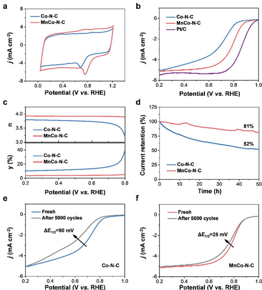
Fig. 4 Electrochemical measurements of MnCo-N-C and controls. (a and b) CV and LSV curves obtained in  $O_2$ -saturated electrolytes, respectively. (c) Electron transfer number ( $n$ ) and  $H_2O_2$  yield ( $y$ ), and (d) the  $i-t$  experiments of catalysts, respectively. (e and f) LSV curves of catalysts before and after 5000 cycles of tests, respectively.
