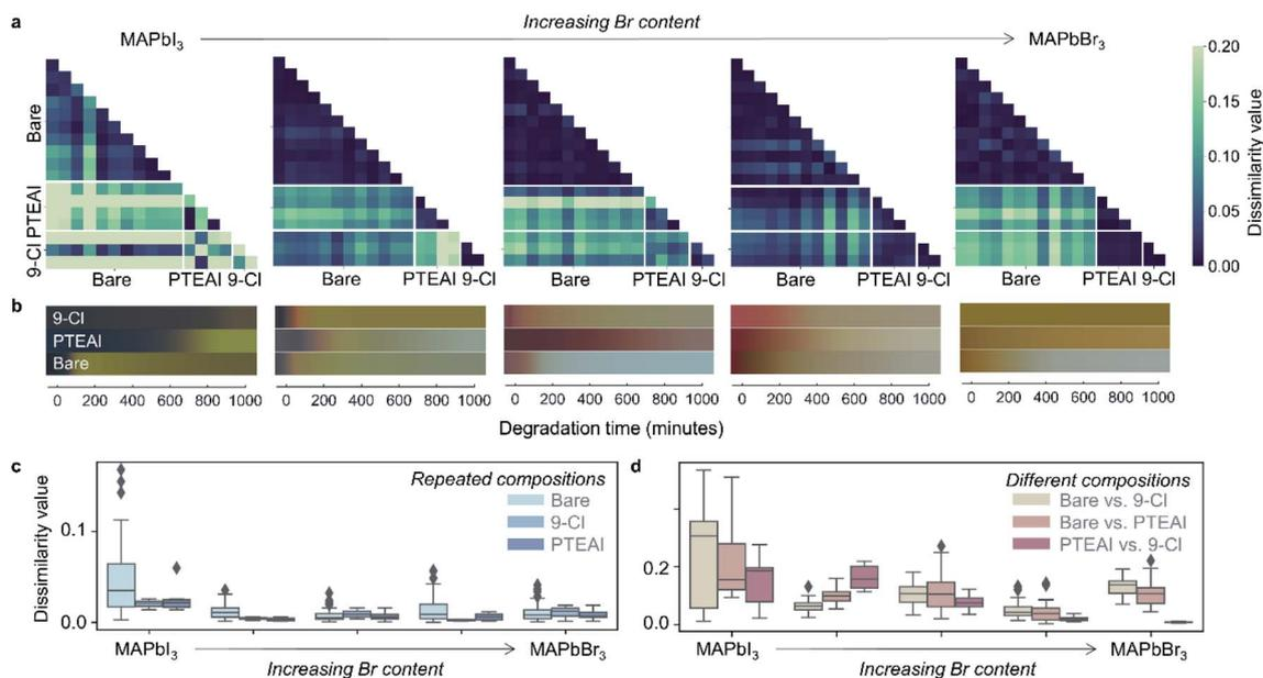
Fig. 2 The dissimilarity matrix of degradation films' color change over time. (a) The dissimilarity matrices (for  $t = 999$  minutes) using cosine distance measure, (b) the degradation film color change of bare, PTEAI-capped, and 9-Cl-capped mixed-halide absorber ( $\text{MAPb}(\text{I}_{0.75}\text{Br}_{0.25})_3$ ) films during degradation, and the boxplot summary of dissimilarity values for (c) repeated compositions and (d) different compositions.
