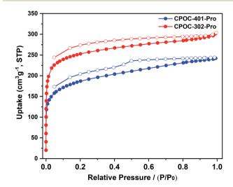
Fig. 4 N<sub>2</sub> sorption isotherms of CPOC-401-Pro and CPOC-302-Pro at 77 K.
