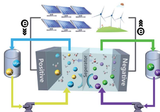
Fig. 1 A schematic diagram of a VFB.
