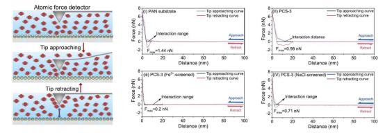
Fig. 12 Schematic diagrams showing measurements of the interaction between PIP and the substrate with an atomic force detector and forcedistance curves for wetting of substrate surfaces. The atom-scale PIP-monomer interactions with PAN(i), PCS-3 (ii), PCS-3 (Fe<sup>3+</sup>-screened) (iii), and PCS-3 (NaCl-screened) (iv) were measured [reprinted with permission from ref. 162. Copyright 2021, Elsevier].
