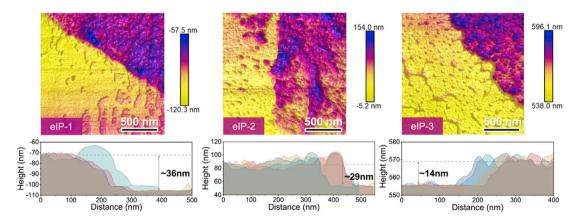
Fig. 11 AFM images and corresponding height profiles for substrate-free eIP polyamide membranes [reprinted with permission from ref. 162. Copyright 2021, Elsevier].
