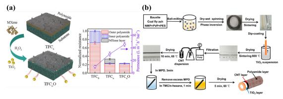
Fig. 4 (a) The MXene lamellar layer was eliminated by mild oxidation after IP to avoid imparting additional hydraulic resistance [reprinted with permission from ref. 17. Copyright 2021, American Chemical Society]. (b) Schematic diagram of the preparation process for a ceramic-based FO membrane with a  $TiO_2/CNT$  nanocomposite interlayer [reprinted with permission from ref. 87. Copyright 2020, American Chemical Society].
