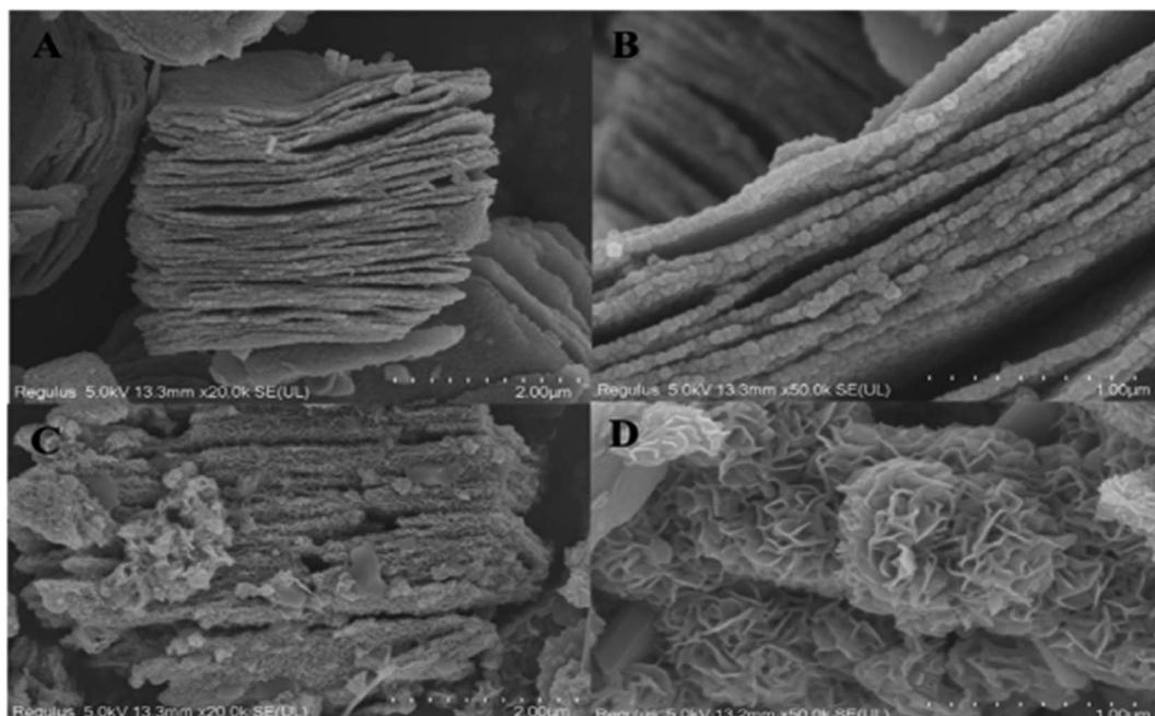
Fig. 8 SEM images of pure  $\text{Ti}_3\text{C}_2$  (A and B) and  $\text{MoS}_2$ - $\text{Ti}_3\text{C}_2$  (C and D).<sup>95</sup>
