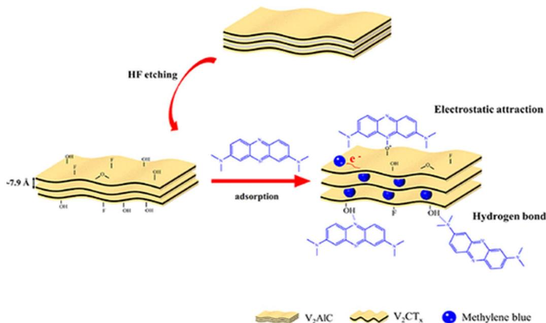
Fig. 10 Mechanism of adsorption of MB on  $V_2CT_x$  MXene surface.<sup>117</sup>
