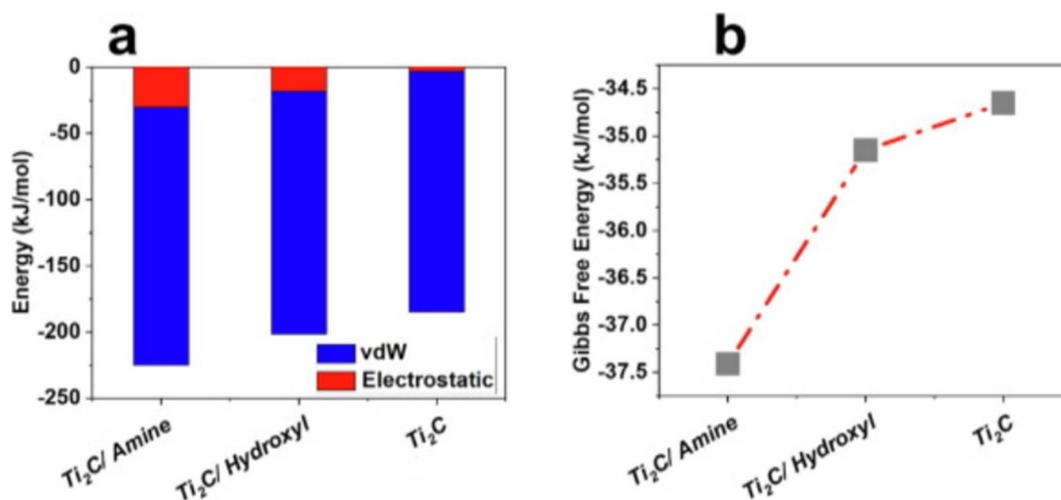
Fig. 6 (a) Gibbs free energy and (b) adsorption energy profiles after the interaction of cloxacillin with functionalized  $Ti_2C$  (vdW = van der Waals interaction).<sup>62</sup>
