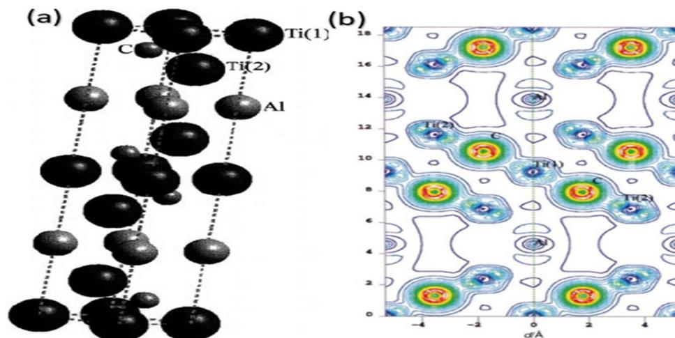
Fig. 2 (a) Crystal assembly and (b) charge density distribution pattern of  $\text{Ti}_3\text{AlC}_2$ .<sup>25</sup>
