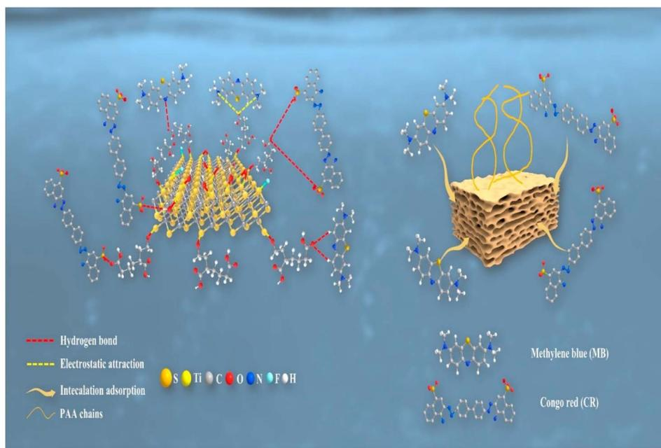
Fig. 9 Graphical representation of adsorption mechanism of AA2-alk-MXene on MB and CR.<sup>87</sup>
