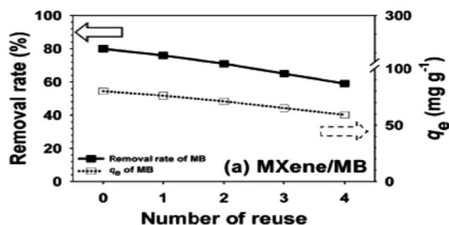
Fig. 11 Reusability performance of MXene's for the adsorption of MB.<sup>115</sup>
