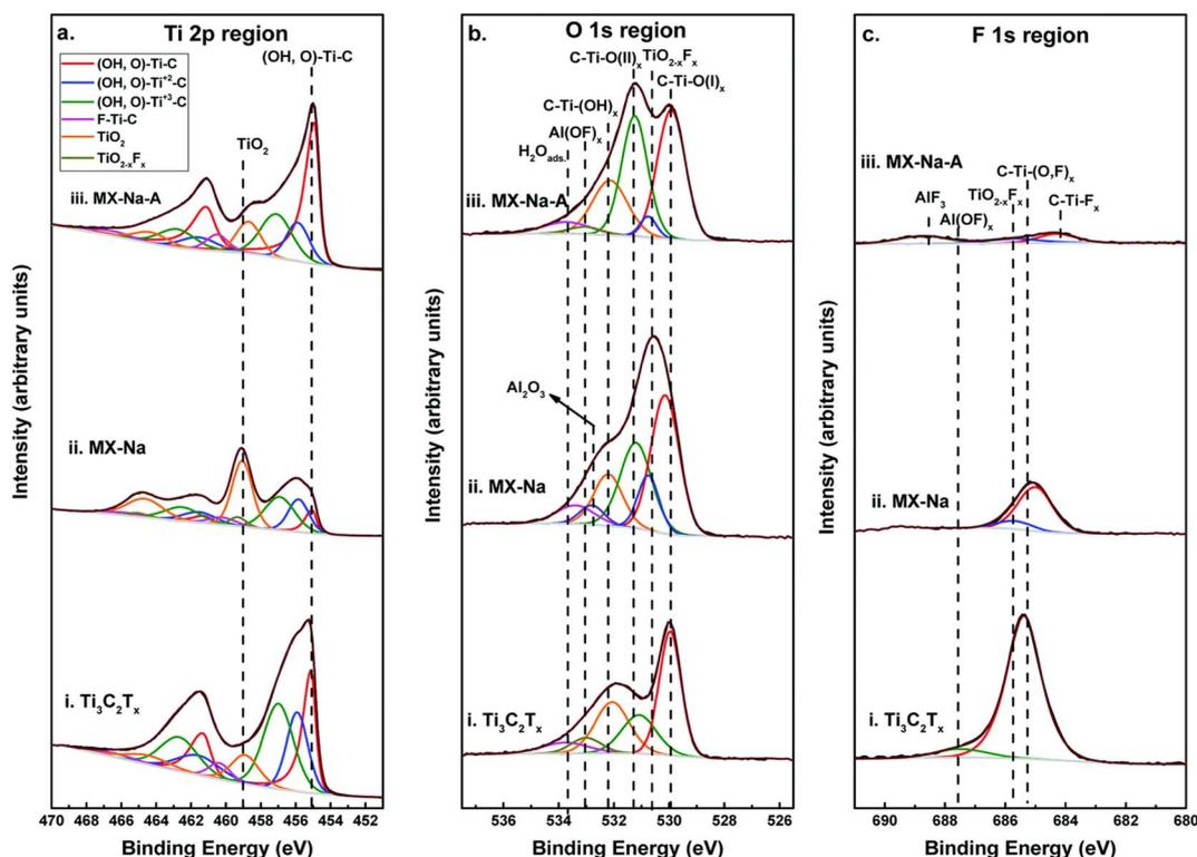
Fig. 5 XPS spectra with curve-fitting for (a) Ti 2p region for (i)  $\text{Ti}_3\text{C}_2\text{T}_x$ , (ii) MX-Na (iii) MX-Na-A. (b) O 1s region for (i)  $\text{Ti}_3\text{C}_2\text{T}_x$ , (ii) MX-Na (iii) MX-Na-A. (c) F 1s region for (i)  $\text{Ti}_3\text{C}_2\text{T}_x$ , (ii) MX-Na (iii) MX-Na-A.<sup>55</sup>
