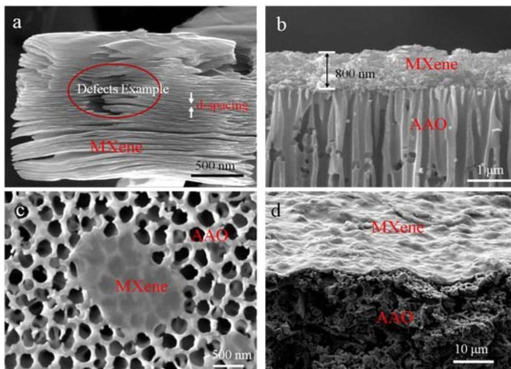
Fig. 4 (a and b) SEM images of cross-section of  $\text{Ti}_3\text{C}_2\text{T}_x$  (c) Top view and (d) low magnification cross section.<sup>47</sup>
