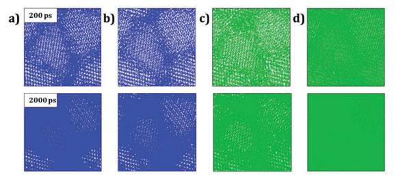
Fig. 4 Trajectory density map of (a)  $\text{Li}_3\text{OCI}$ , (b)  $\text{Li}_3\text{OBr}$ , (c)  $\text{Na}_3\text{OCI}$  and (d)  $\text{Na}_3\text{OBr}$  compounds after 200 ps (top images) and 2000 ps (bottom images). Blue and green lines represents the Li and Na trajectory lines, respectively.
