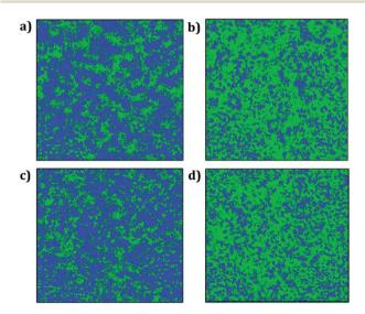
Fig. 8 Trajectory plots of Li and Na in (a)  $Li_2NaOCl$ , (b)  $Na_2LiOCl$ , (c)  $Li_2NaOBr$  and (d)  $Na_2LiOBr$  compounds after 2 ns. Blue and green lines represent the Li and Na trajectory lines, respectively.
