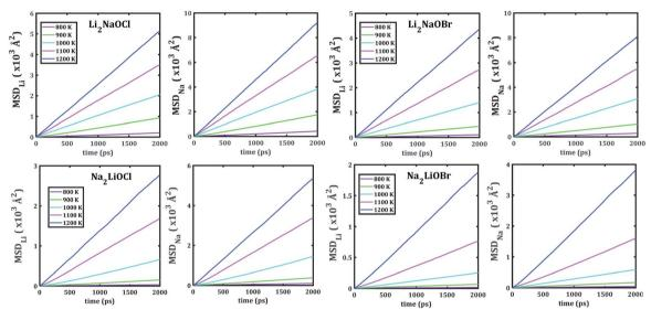
Fig. 5 Li- and Na-mean square displacement (MSD) versus simulation time of Li<sub>2</sub>NaOX and Na<sub>2</sub>LiOX structures.
