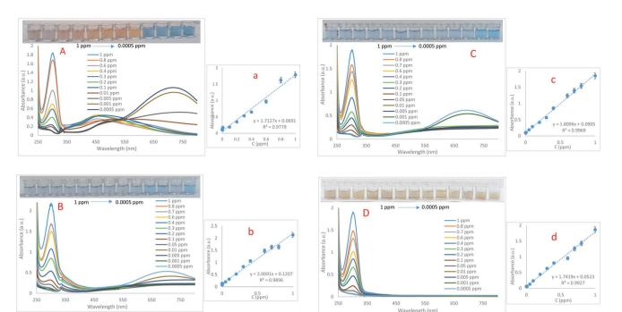
Fig. 2 The UV-Vis spectra of (A) AgNPrs, (B) Cys-capped AgNPrs, (C) Met-capped AgNPrs and (D) AgNWs sensing probes and calibration curves in the presence of various concentration of arsenic (0.0005, 0.001, 0.005, 0.01, 0.05, 0.1, 0.2, 0.3, 0.4, 0.6, 0.7, 0.8 and 1 ppm).
