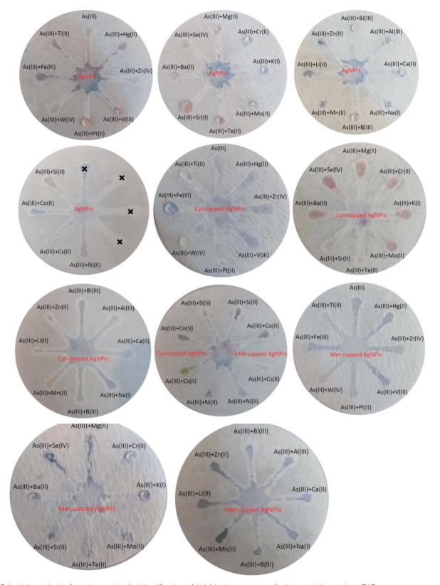
Fig. 4 Selectivity analysis of sensing probes for identification of As( $\parallel$ ) in the presence of other metal ions using  $\mu$ PADs.
