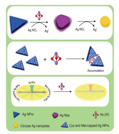
Scheme 1 Schematic illustration of naked-eye detection of As(III) by colorimetric assay based on AgNPs
