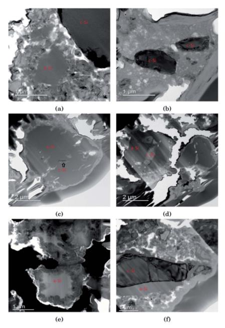
Fig. 3 Bright field TEM images after the first cycle in (a) LiFSI and (b) LiPF<sub>6</sub> (c) after 10 cycles in LiFSI and (d) LiPF<sub>6</sub> (e) high angle annular dark field scanning transmission electron microscopy image of LiFSI after 50 cycles and (f) bright field TEM image of LiPF<sub>6</sub> after 50 cycles.
