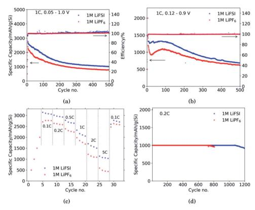
Fig. 1 Galvanostatic cycling tests comparing half cells with 60 wt% Si electrodes cycled in 1 M LiFSI (blue) or 1 M LiFF<sub>6</sub> (red). (a) Galvanostatic cycling in voltage range 0.05-1.0 V, (b) galvanostatic cycling in voltage range 0.12-0.9 V, (c) rate capability in voltage range 0.05-1.0 V, (d) galvanostatic cycling at 0.2C with lithiation of silicon limited to 1000 mA h g<sup>-1</sup> and delithiation to 1.0 V.
