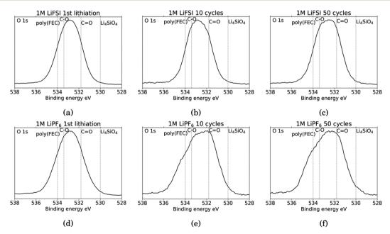
Fig. 6 O 1s spectra for Si electrodes cycled to 1st lithiation, cycle 10 and cycle 50 in LiFSI (a-c) respectively, and in LiPF<sub>6</sub> (d-f) respectively.
