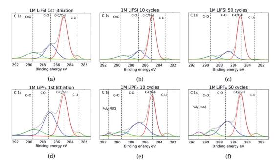
Fig. 7 C 1s spectra for Si electrodes cycled to 1st lithiation, cycle 10 and cycle 50 in LiFSI (a-c) respectively, and in LiPF<sub>6</sub> (d-f) respectively.
