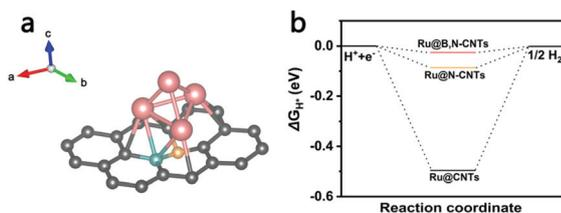
**Fig. 7** (a) Optimized structures of H\* adsorbed on an Ru cluster anchored on a boron and nitrogen-doped carbon layer model. The ruthenium, boron, nitrogen and carbon atoms are pink, blue, yellow and grey, respectively. (b) The HER free energy diagram.  $\Delta G_{H^*}$  is calculated at the equilibrium potential of different models.
