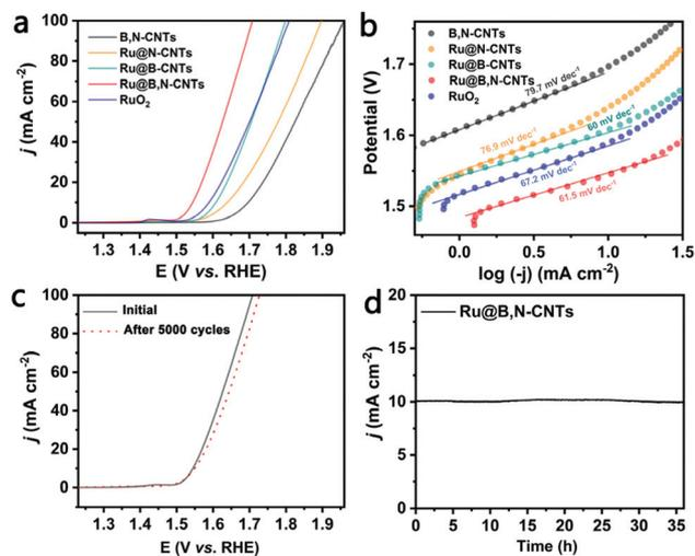
**Fig. 5** (a) The linear sweep voltammetry (LSV) curves for the OER of the B,N-CNTs, Ru@B-CNTs, Ru@N-CNTs, and Ru@B,N-CNTs, and commercial RuO<sub>2</sub> in 1 M KOH solution. (b) The corresponding Tafel plots for the electrocatalysts. (c) The LSV curves obtained for OER over Ru@B,N-CNTs before and after 5000 cycles of CV scans. (d) The chronoamperometric *i*–*t* curve of the Ru@B,N-CNTs for 36 h.
