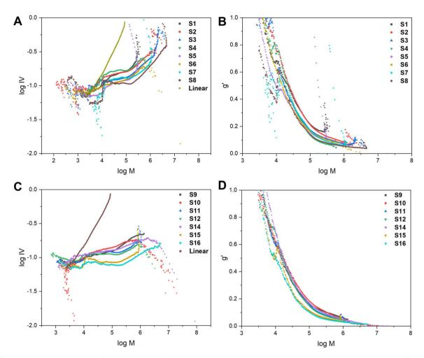
Fig. 4 The Mark-Houwink plots and g' vs. log M plots for the core-crosslinked branched polymers formed with a bis-methacrylate (A and B) and bis-thiomethacrylate (C and D) crosslinkers.
