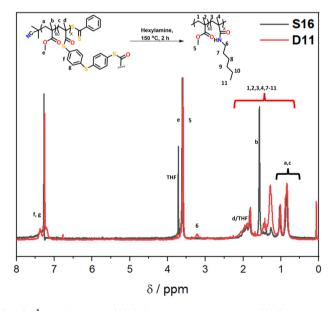
Fig. 6  $\,^{1}$ H NMR spectra (CDCl $_{3}$ ) of the starting polymer (S16) and crude hexylamine degraded product (D11), showing the formation of the amide product.
