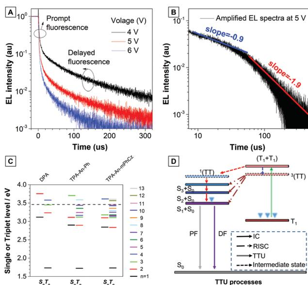
Fig. 5 (A) Transient EL decay of the non-doped device B2 at different voltages. (B) Amplified EL spectra of the non-doped device B2 at 5 V. (C) Energy diagrams. Energy levels and twice the  $T_1$  energies (dashed line) of the anthracene derivatives calculated using B3LYP/6-311G(d,p), where  $n$  is the quantum number used to indicate the excited state. (D) Proposed TTU mechanism based on the emitters.
