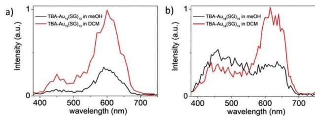
Fig. 15 Two-photon excited fluorescence spectra for (a) TBA- $\text{Au}_{15}(\text{SG})_{13}$  and (b) TBA- $\text{Au}_{18}(\text{SG})_{14}$  at the excitation wavelength of 780 nm. Reproduced with permission.<sup>180</sup> Copyright 2018. Wiley-VCH.
