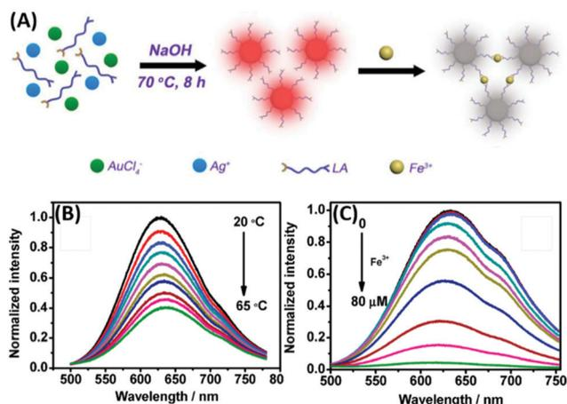
Fig. 22 Schematic illustration of the (A) synthesis of lipoic acid-stabilized Au/Ag BMNCs and their  $\text{Fe}^{3+}$  sensing and (B) temperature- and (C)  $\text{Fe}^{3+}$ -dependent fluorescence quenching. Reproduced with permission from ref. 209, Copyright Elsevier (2016).
