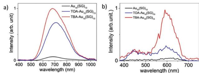
Fig. 14 One-photon excited fluorescence spectra of  $\text{Au}_{15}(\text{SG})_{13}$  in (a) water and (b) presence of bulky ammonium cations, namely, tetrabutylammonium (TBA) and tetraoctylammonium (TOA) for (TOA- $\text{Au}_{15}(\text{SG})_{13}$  and TBA- $\text{Au}_{15}(\text{SG})_{13}$  in methanol). Reproduced with permission.<sup>180</sup> Copyright 2018. Wiley-VCH.
