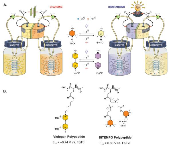
Fig. 1 (A) Illustrative design of polypeptide-based redox flow battery during charging and discharging. (B) Molecular structures of the redox-active polypeptides.
