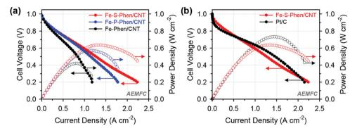
Fig. 5 Alkaline AEMFC performance of MEAs using (a) Fe-Phen/CNT, Fe-P-Phen/CNT, and Fe-S-Phen/CNT as cathode catalysts and (b) Fe-S-Phen/CNT. CNT and Pt/C as cathode catalysts. Reproduced from ref. 76 with permission from the American Chemical Society
