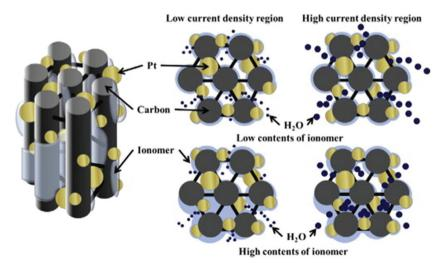
Fig. 4 Schematic illustration of the effect of ionomer contents in the low and high current density regions. Reproduced from ref. 61 with permission from Elsevier B.V.
