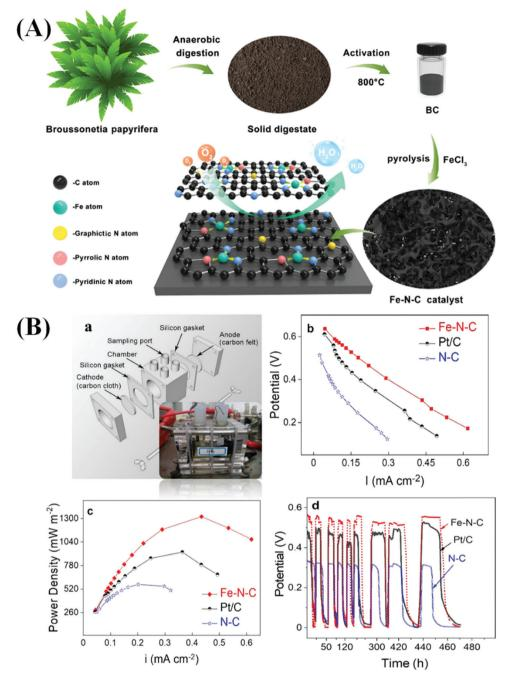
Fig. 7 (A) Schematic illustration of the fabrication of hierarchical Fe-N-C catalysts derived from the solid digestate. (B) Schematic illustration of a singlechamber MFC (a); power density (b) and electrode polarization curves (c), and the periodic variation of single-chamber MFCs coupled with the Fe-N-C, Pt/C, and N-C catalysts (d). Reproduced from ref. 133 with permission from the American Chemical Society
