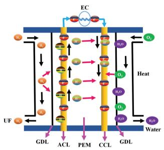
Fig. 3 The working principle of PEMFCs (note:  $H_2$  – hydrogen,  $O_2$  – oxygen,  $H_2O$  – water, UF – unused fuel, GDL – gas diffusion layer, ACL – anode catalyst layer, PEM - proton exchange membrane, CCL - cathode catalyst layer, H<sup>+</sup> - proton, e<sup>-</sup> - electron).
